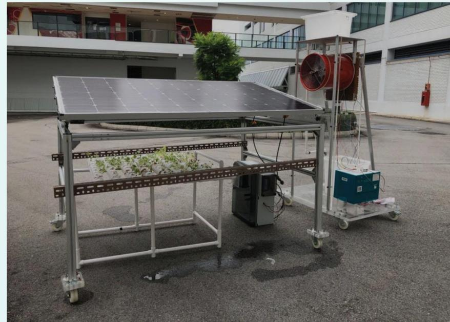
Hydroponics system under the solar panel, evaporative cooling at the side and a IP66 circuit box to protect the circuit from weather conditions.
